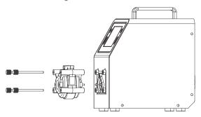
**Multi-stage connection:** When multiple pump heads are connected in series, the extension screw is used to connect, and the pump head shaft of the former pump head can be embedded in the connection hole of the latter pump head.
